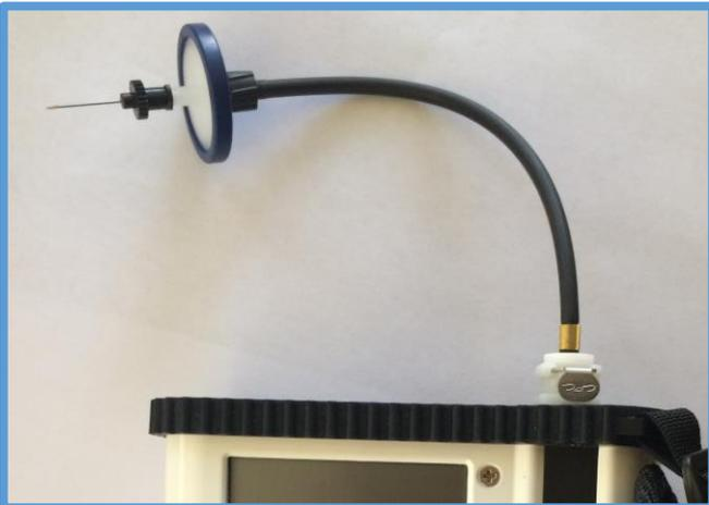
After the start button has been pressed, the pump will run until the sample volume (default: 15 mL) has been drawn into the F-950, and then the loop will close while the sample is analyzed. Maximum sample volume in fixed volume mode is 18.5 mL. Minimum sample volume is 10 mL for 5-10% accuracy.
